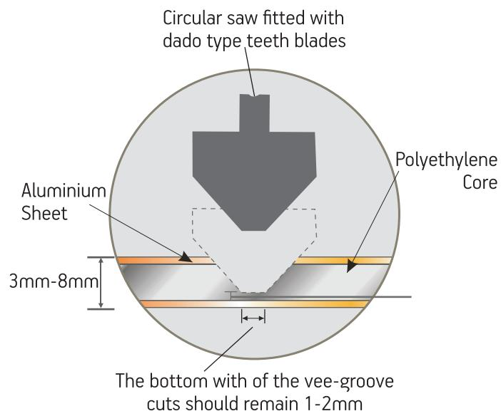
The thickness of the remaining polyethylene core to the aluminium sheet should remain approximately 0.3 - 0.5 mm
